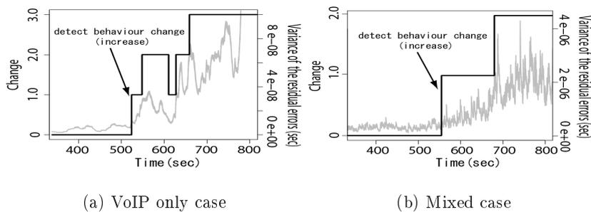
**Fig. 7.** Simulation results of automatic change detection
