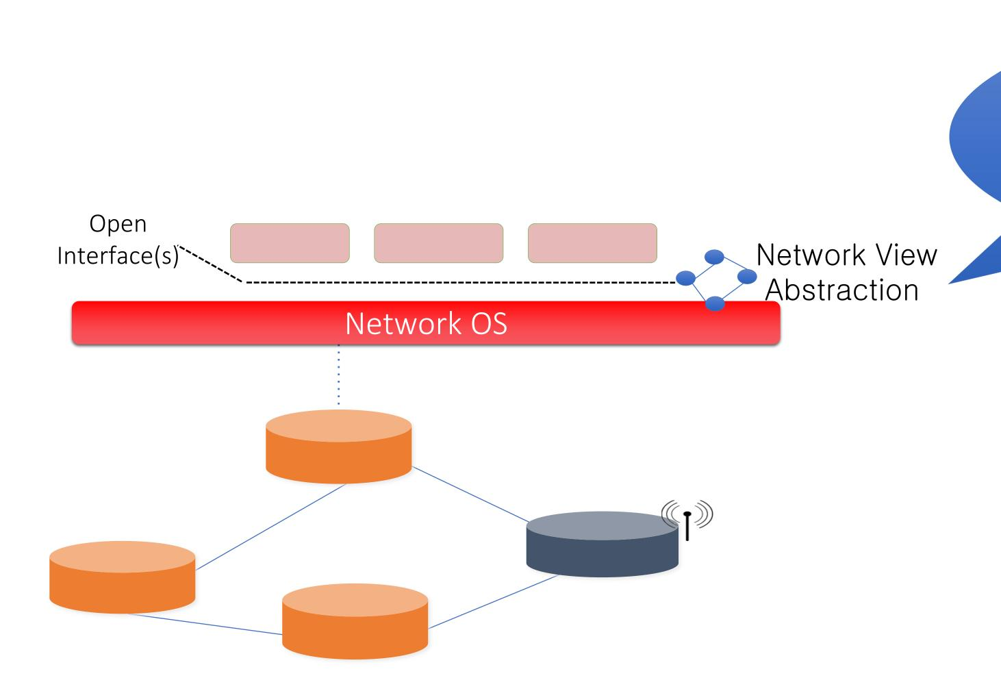
Makes it easy to write control, config, sensing apps: locally manipulate graph
