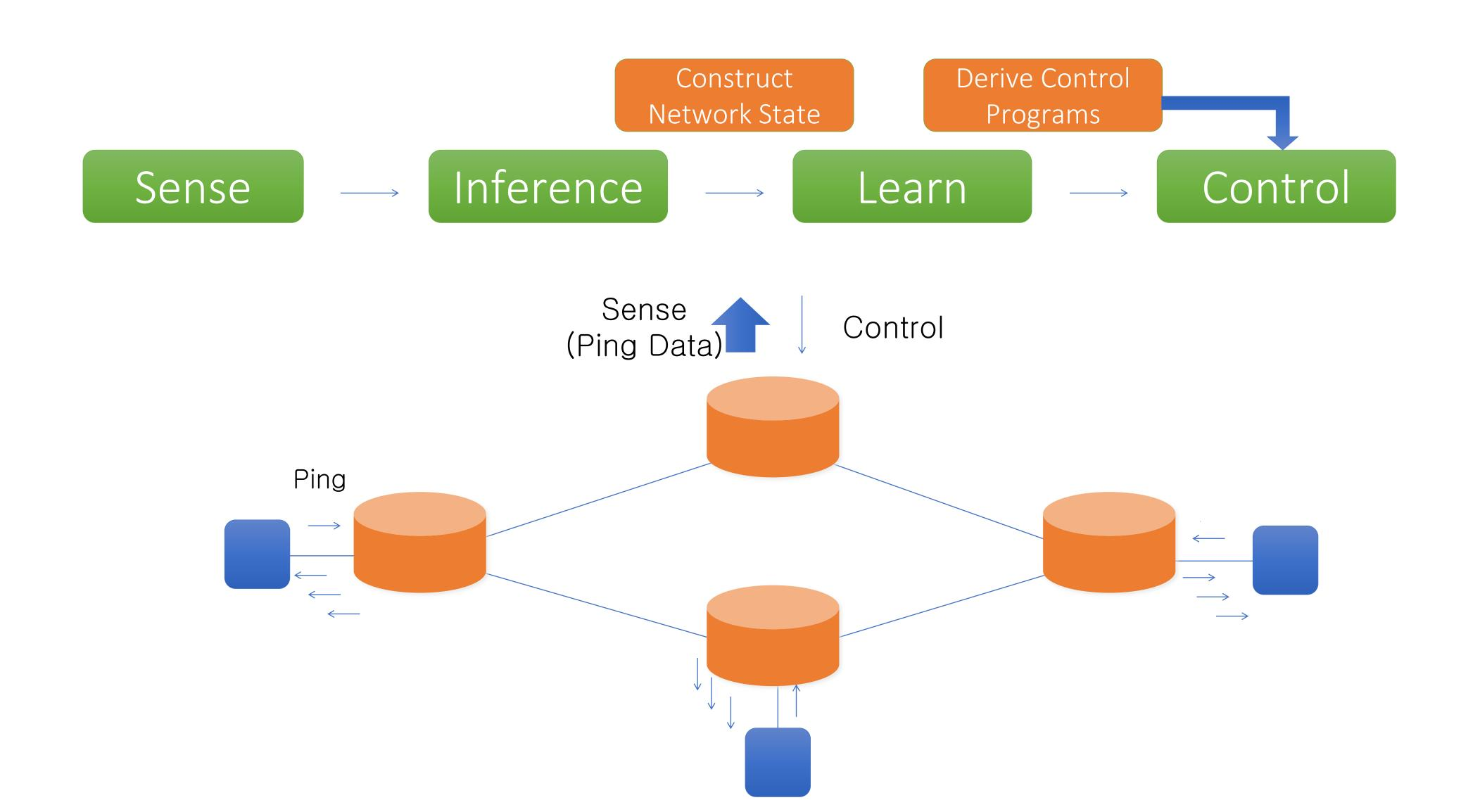
Software defined networks make it much easier and efficient to do sensing and control
