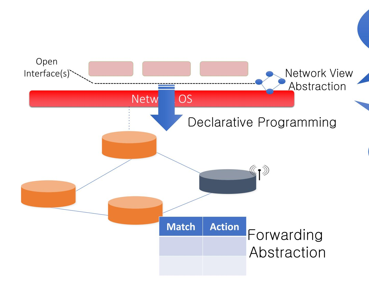
Makes it easy to write control, config, sensing apps: locally manipulate graph
