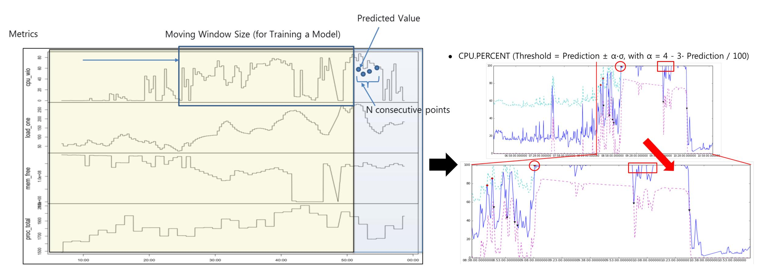
**Anomaly Detection using dynamic threshold**
