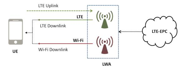
• The LWIP aggregation technique involves the use of IPsec tunnels to provide LTE-WiFi aggregation, without making any major changes to the wireless local area network (WLAN) infrastructure.
