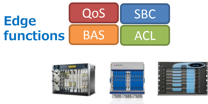
Edge routers (dedicated hardware)
