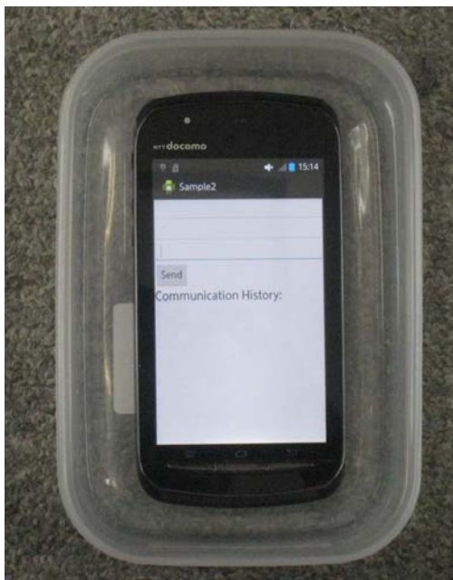
Android Smartphone IEEE 802.11g 100bytes / 500bytes 1s interval Auto bitrate (5-54Mbps)
